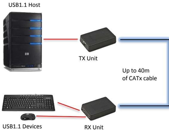
The CrystalLink USB1.1 Dual-Port is ideal for use in commercial or industrial environments, or in a computer room where USB devices need to be connected at short distances away from a host PC.
