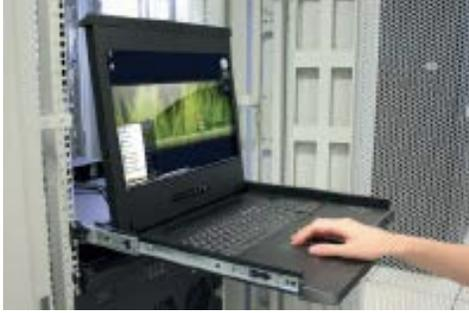
**Installation** RackView High-Res is very easy to install. Simply adjust the rack-rail length to the depth of your rack, slide the unit through the rack and secure the rack mount brackets to the front and rear rack rails.
