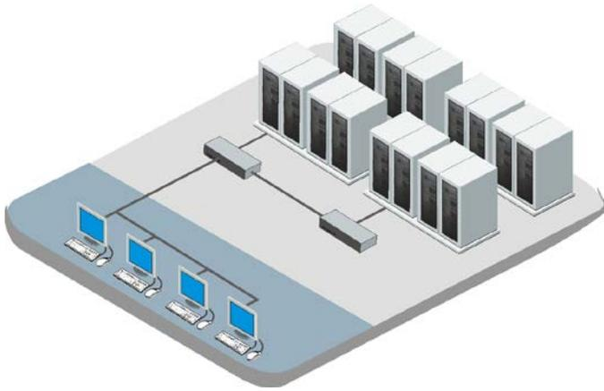
**Models** UltraMatrix E-Series switches are available in several models. They have fixed port configurations and plug-in expansion cards. The 4xE units connect 4 users with 4, 8 or 16 computers. The 2xE units connect 2 users with 4, 8, or 16 computers. The E-Series switches can be connected together giving access to as many as 1000 CPUs.
