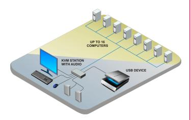
Installation Installing the UltraView DVI consists of connecting up to 16 DVI computer video sources to the video inputs along with their associated USB inputs and stereo audio outputs. Attach the user's monitor, keyboard and mouse, USB 2.0 peripherals, and stereo speakers to the console connectors. Apply power to the monitor and the switch, then apply power to the computers.
