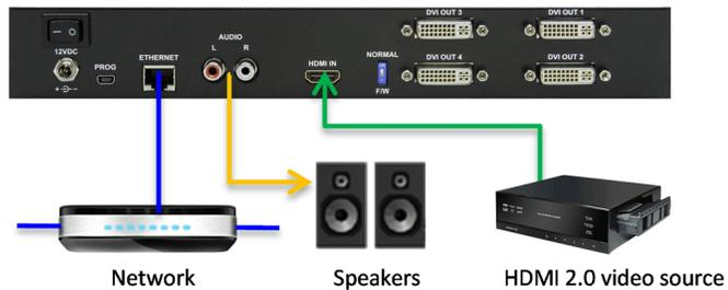
**Overview** The UltraVista 4K Video Wall accepts either HDMI or DVI input. It supports four HD DVI or HDMI outputs, each of which can be individually configured.
