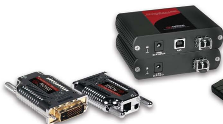
CrystalView DVI Micro Single-link DVI over single fiber
