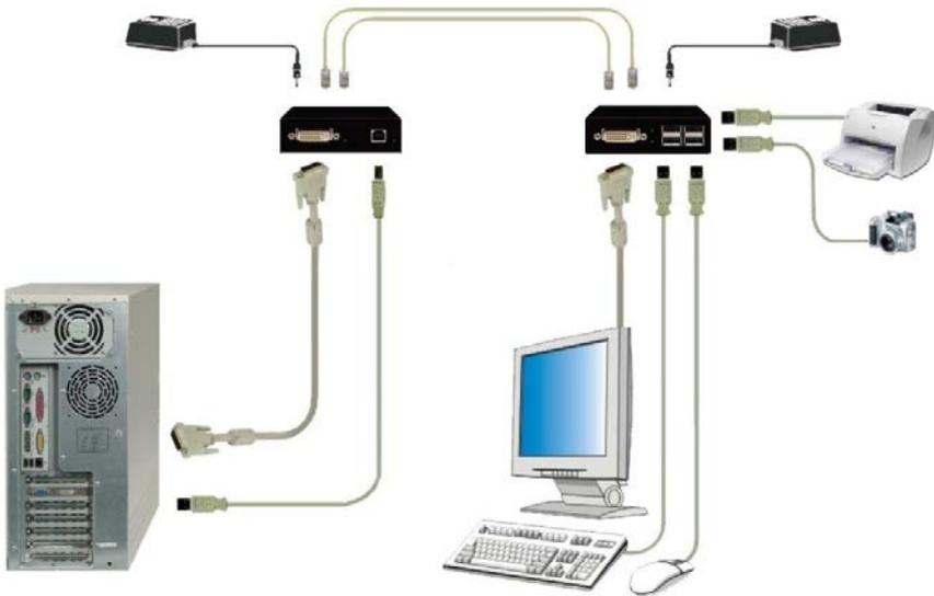
Figure 7. Single head Installation (USB-2.0)
