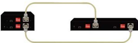
CATx cabling is connected as shown to the left. Up to 150 ft. max.
