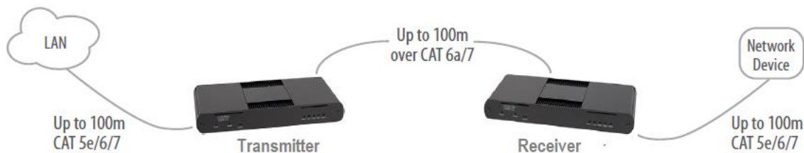
Figure 3. Ethernet LAN Connections
