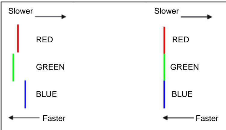
Figure 10. Color skew delay compensation
