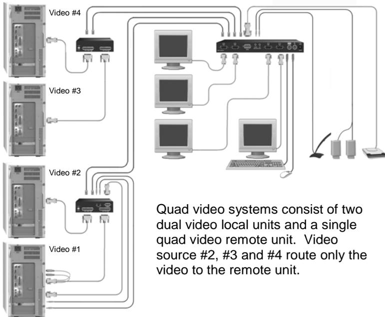
Quad video systems consist of two dual video local units and a single quad video remote unit. Video source #2, #3 and #4 route only the video to the remote unit.
