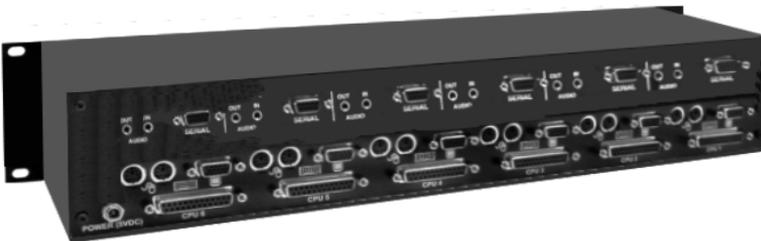
6-DB25 – CPU/KVM connections    6-DB9 serial connectors
