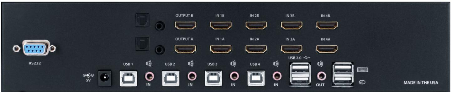
Figure 2. MultiVideo HDMI Dual Rear Panel
