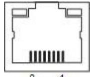
Figure 88. I/O Port RJ45 Connector Pinouts
