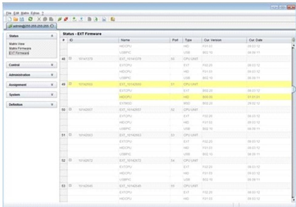
Figure 83. Viewing Firmware Status on the connected Extenders through the Java Tool
