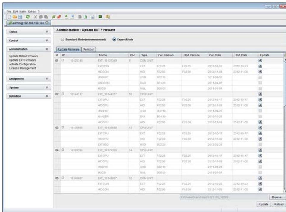
Figure 63. Extender Update in Expert Mode – Step 1 (from the Java Tool)
