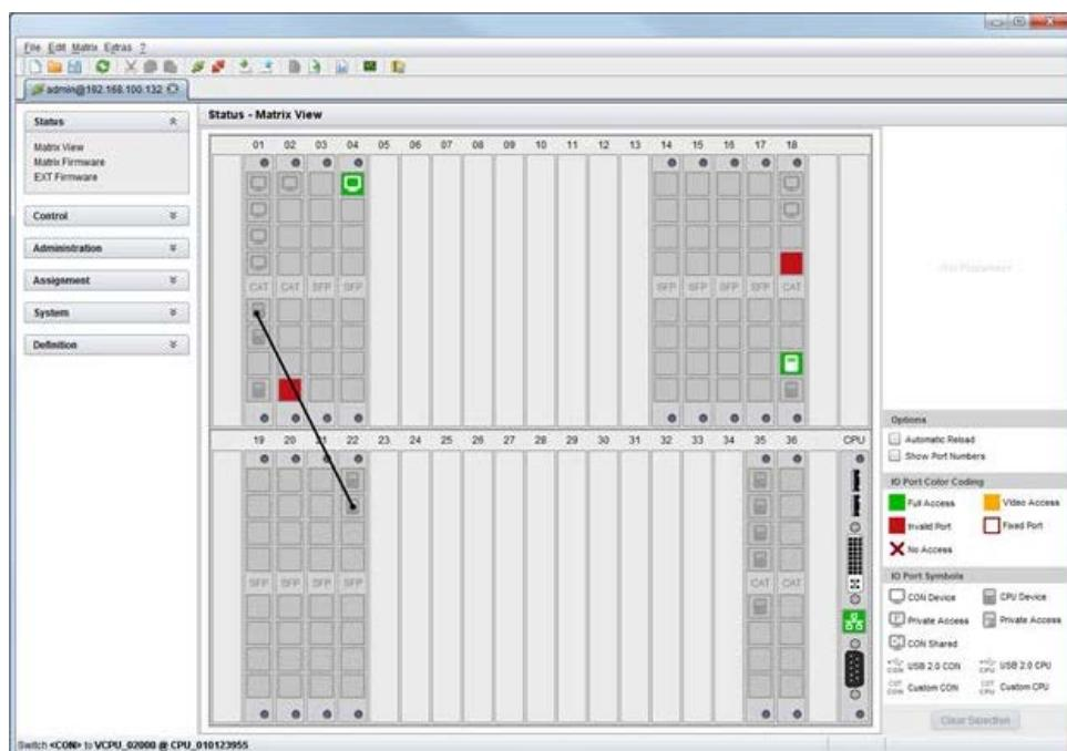
Figure 69. Extended KVM Switching through Java Tool - Method 2 (from Matrix View Option)
