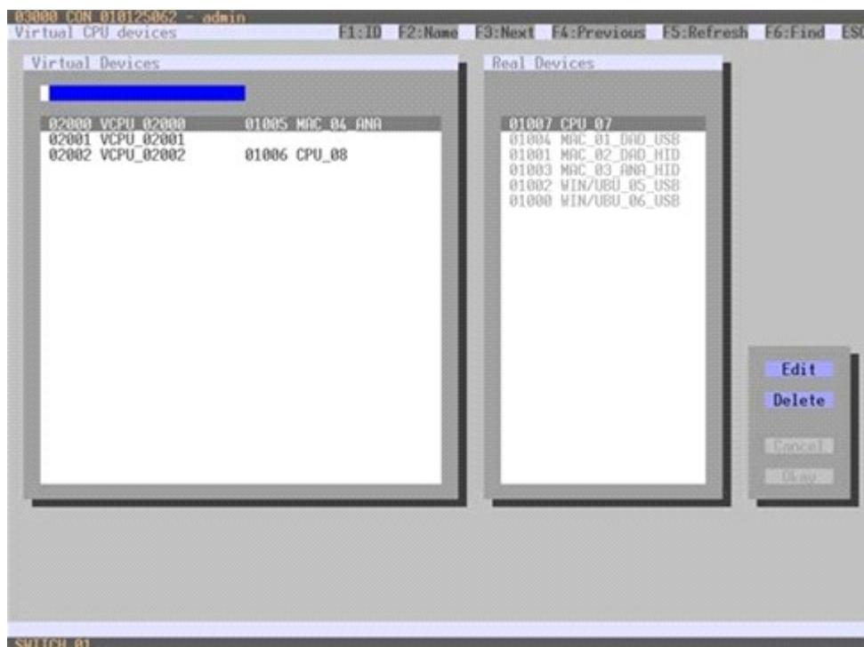
Figure 17. Virtual CPU Devices Assignment through OSD
