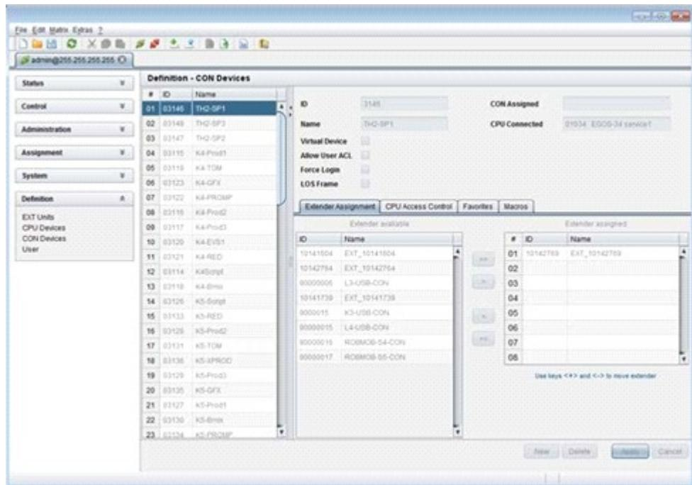
Figure 43. Setting up CON Devices through the Java Tool
