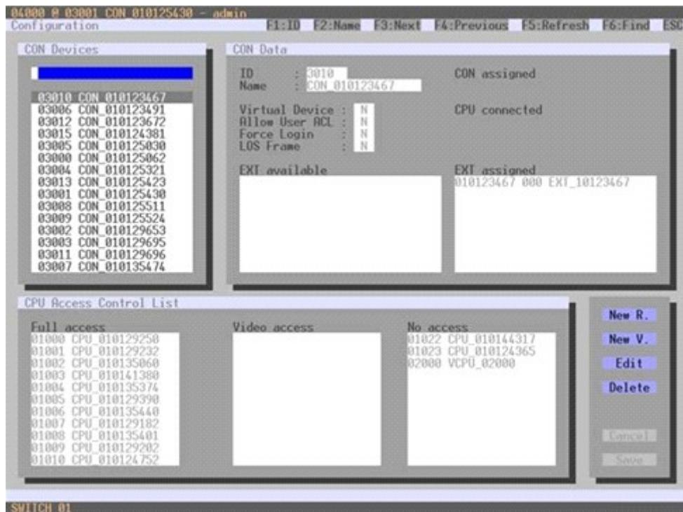
Figure 42. Setting up CON Devices through OSD
