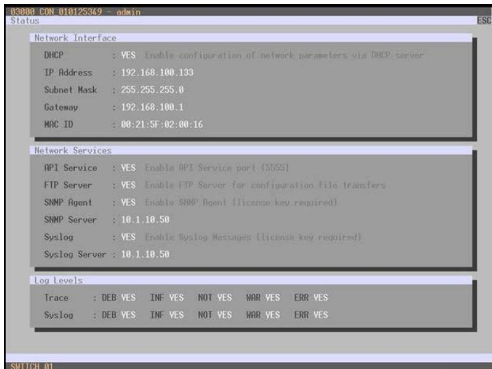
Figure 79. Viewing Network Status through OSD
