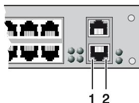
Figure 72. LAN Port Status LEDs
