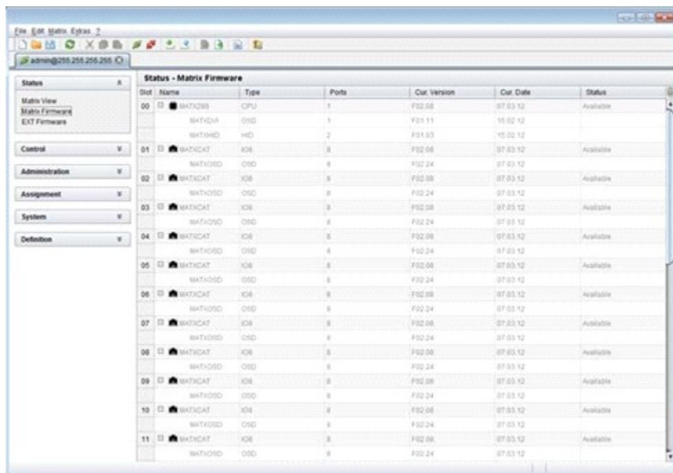
Figure 82. Viewing Firmware Status through the Java Tool
