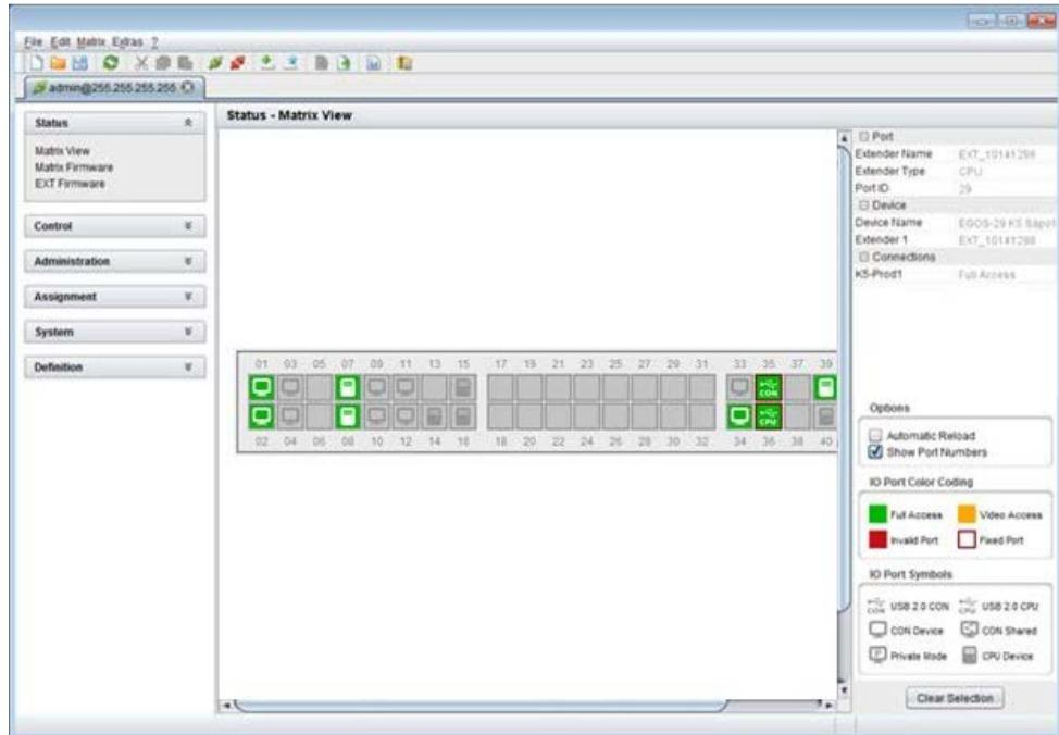
Figure 77. Viewing Port Status with the Java Tool (Example 2)
