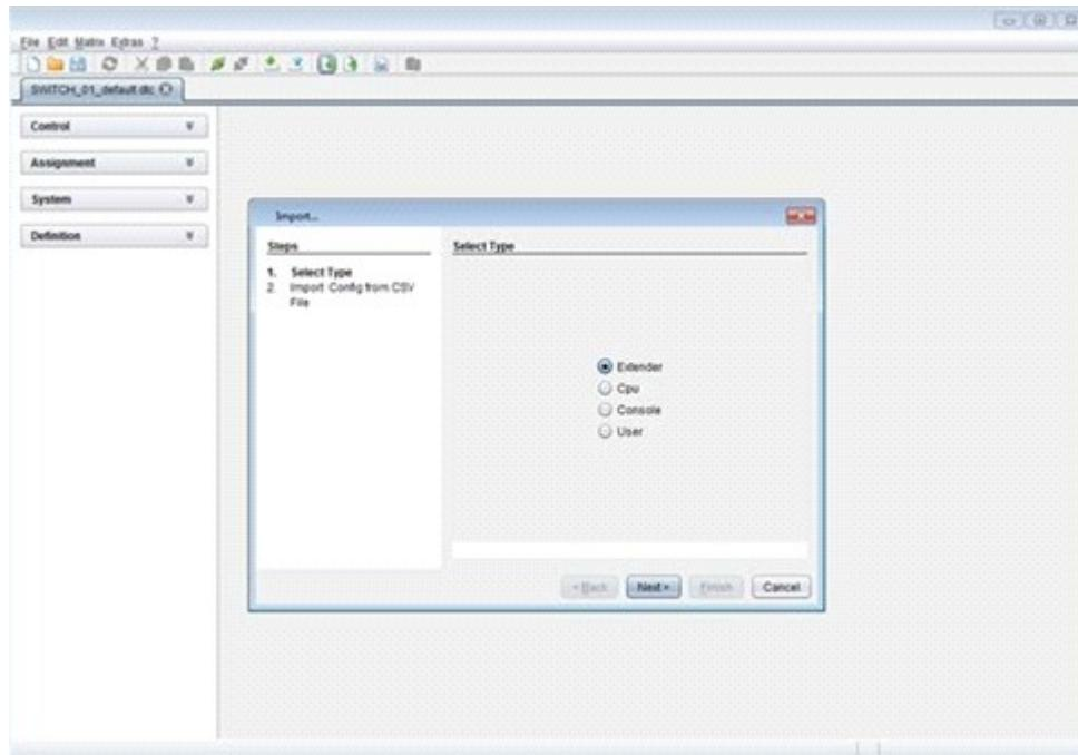
*Figure 59. Importing Configuration Lists through the Java Tool*
