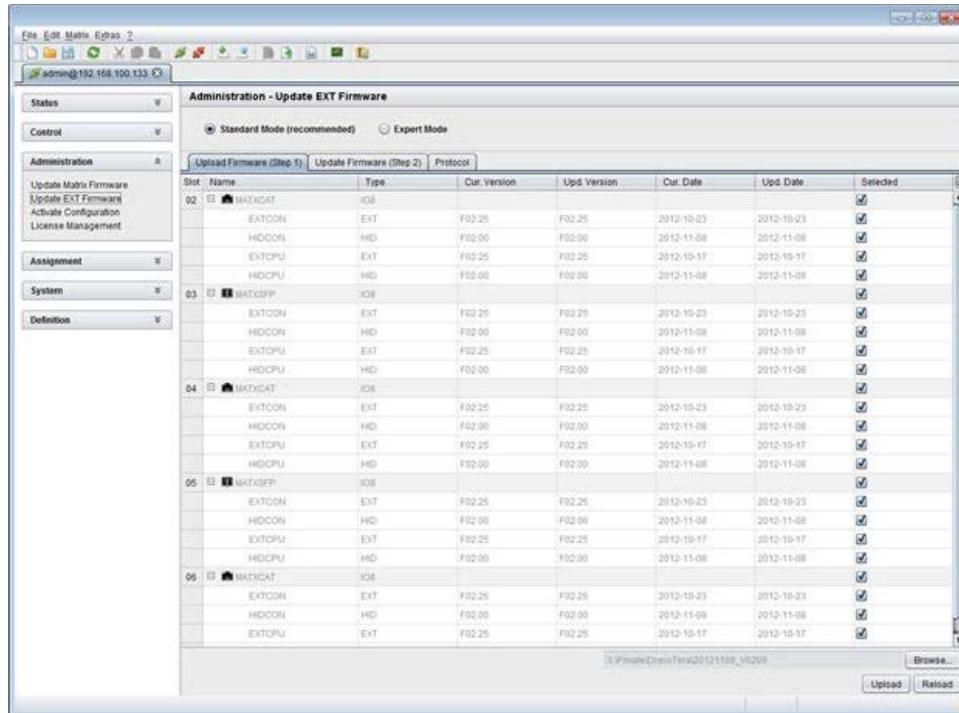
Figure 61. Extender Update in Standard Mode through the Java Tool - Step 1 (Upload Firmware)
