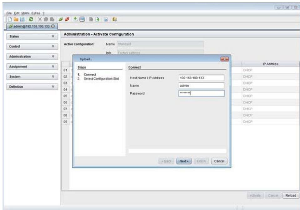
Figure 53. Saving internal configuration through the Java Tool
