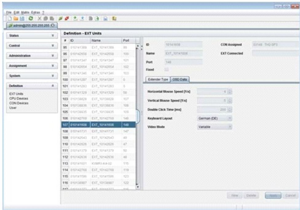
Figure 45. Modifying Mouse and Keyboard Settings through the Java Tool
