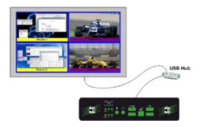
7. Connect the mouse and keyboard devices to the USB hub.
