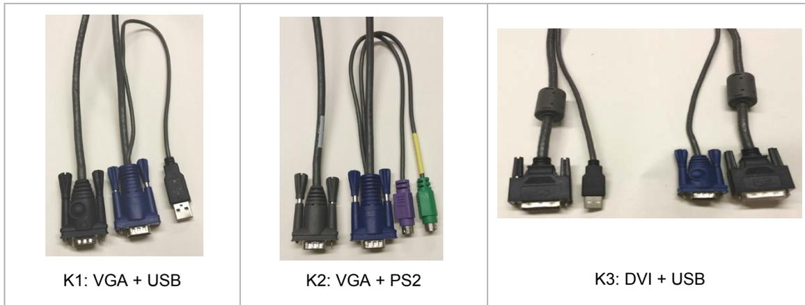
**Figure 8. RackView device interface cables**
