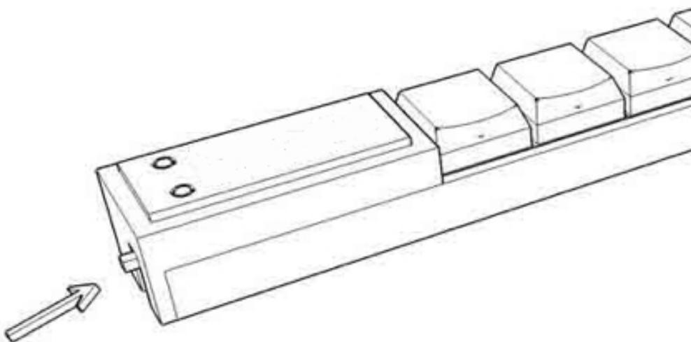
The programming switch is located on the left side edge of the 4/8/16 Keystick. The program switch will display the MacroWorks GUI by default. If desired, the program switch can be used like any other key on the RCK-Keystick, effectively making it a 25 button device.
