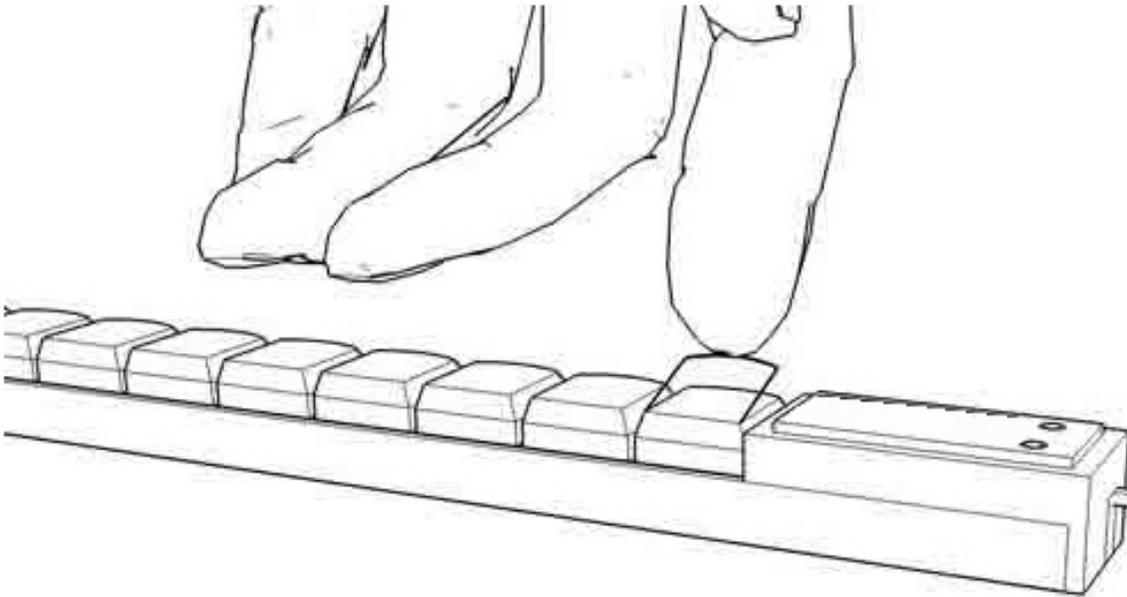
Labels may be inserted under the clear lens, which can be removed by prying with a fingernail or other thin object. Additionally, custom keycaps and lens are available.
