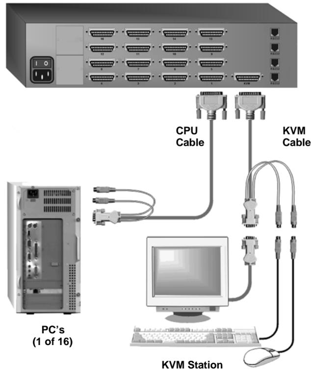
Figure 2. Single Unit configuration
