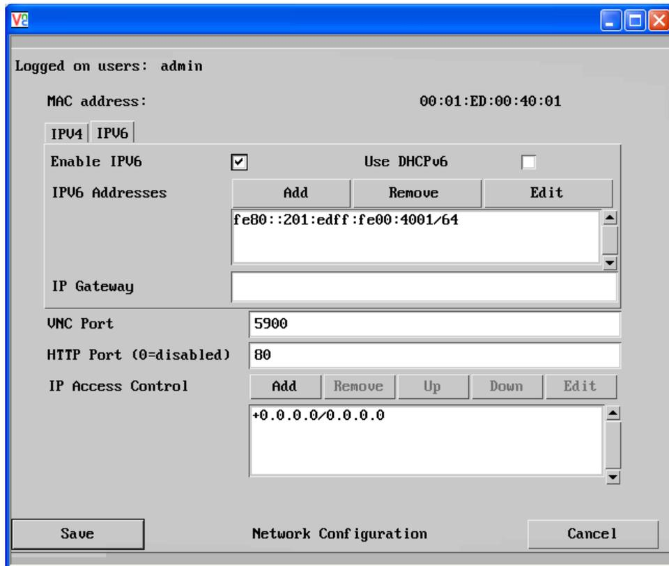
Figure 57. Network Configuration Screen – IPv6
