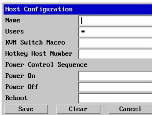
The image shows a 'Host Configuration' dialog box with a blue title bar. It contains several input fields: 'Name' (empty), 'Users' (containing '\*'), 'KVM Switch Macro' (empty), 'Hotkey Host Number' (empty), 'Power Control Sequence' (a section header), 'Power On' (empty), 'Power Off' (empty), and 'Reboot' (empty). At the bottom are three buttons: 'Save', 'Clear', and 'Cancel'.
