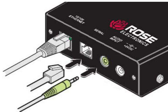
Figure 6. Optional Serial and Audio connections
