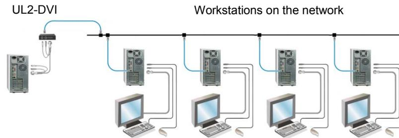
Figure 15. UL2-DVI on the desired network
