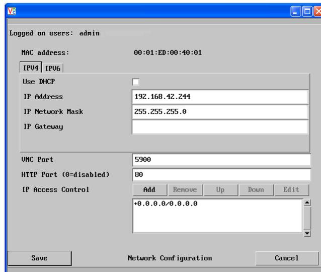
Figure 14. Setting Initial IPv4 network address
