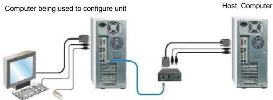
**Figure 9. Connections for initial IP configuration**
