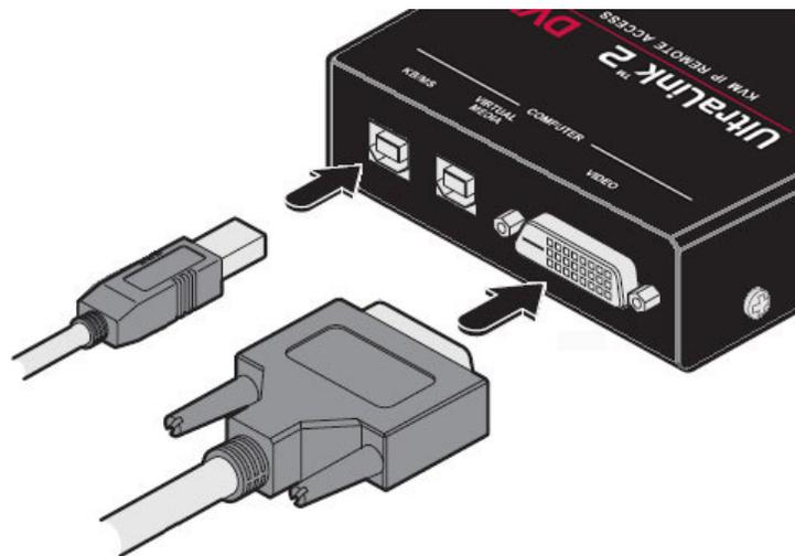
Figure 4. Keyboard/Mouse and DVI connections
