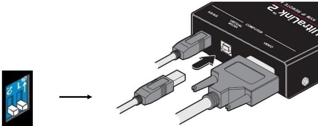
Figure 7. UL2-DVI draws power from 2 USB connections
