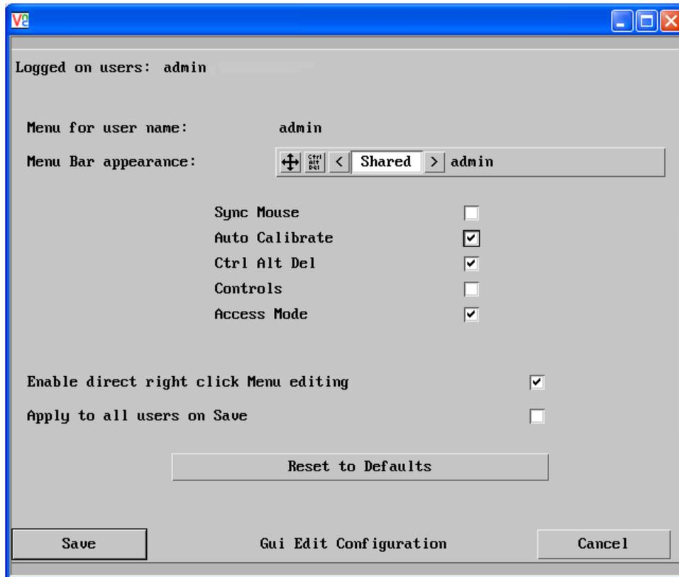
Figure 50. Gui Edit Configuration Screen
