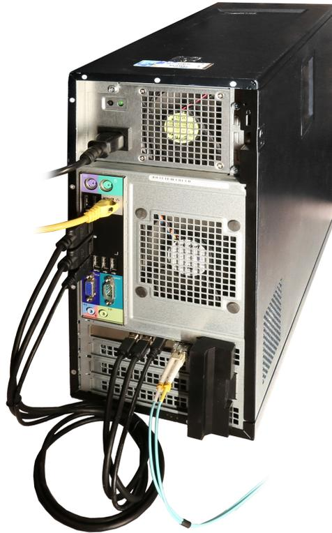
**Figure 21. PCIe 2-port transmitter card with fiber**
