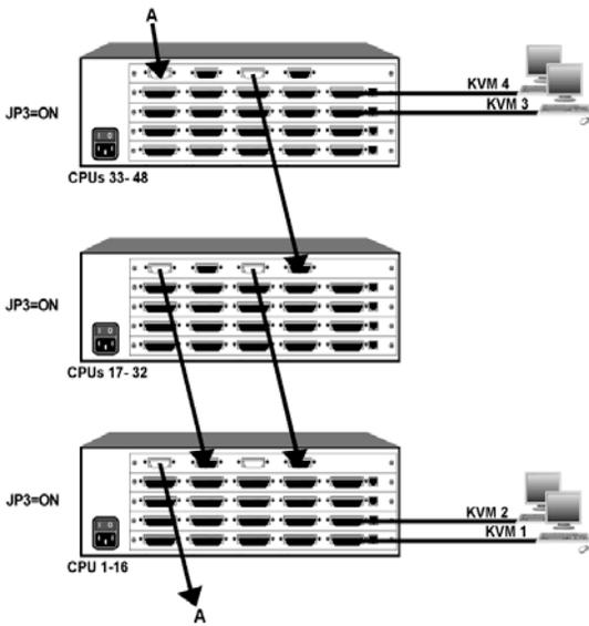
Figure 13. UM4 Staggered BUS
