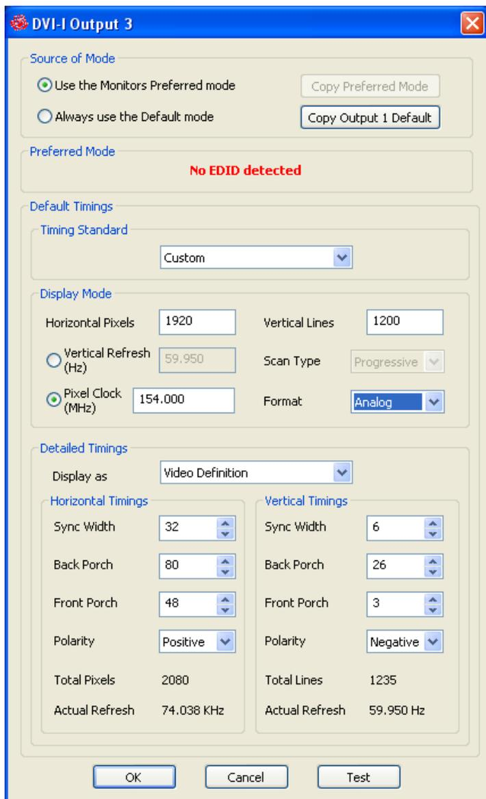
The source of mode selection controls whether the UltraVista Plus output should take its timing values and resolution from the preferred mode of the monitor that is connected, or use its internally programmed 'default' mode. Please note that only the internal default timings can be edited in this dialog.
