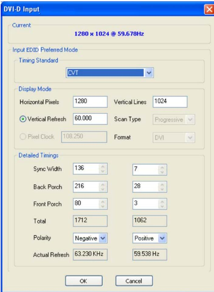
The DVI-D Input dialog displays the resolution of the current mode for reference and allows the timings of the EDID preferred mode to be edited. The dialog supports standard timing formulae such as:
