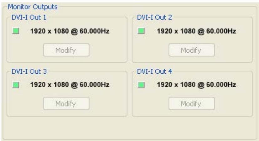
Individual monitor outputs can be configured by clicking on the corresponding Modify button. This will bring up a timing dialog similar to that of the input timings. This dialog is shown below.
