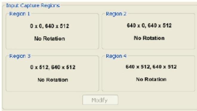
The numbers denote the top, left, width and height coordinates of the region that is to be displayed. Note, these are described in terms of the current active input resolution. If the input resolution changes, the capture region coordinates scale to the new input resolution in order to maintain the same proportions.
