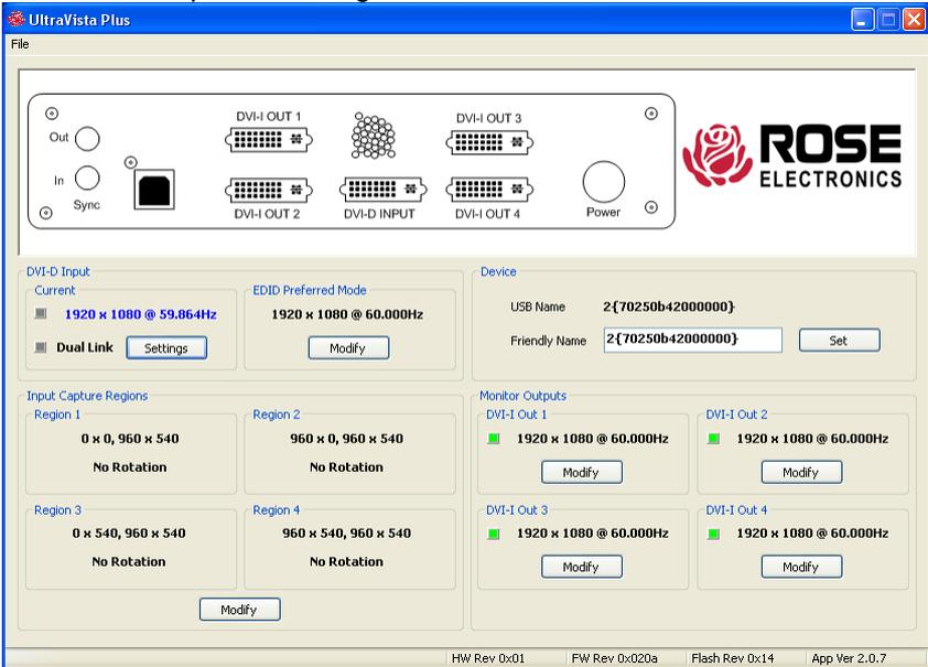
To change the timings of the input EDID click on the Modify button. The following dialog window will be displayed. From this window you can modify the input EDID preferred mode timing standard, the display mode, and detailed timing.
