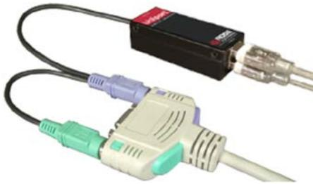
Connect the Uniport's PS/2 keyboard and mouse connectors to the corresponding PS/2 connectors on the KVM cable. Connect the video monitor cable if it was disconnected, to the HD15M connector on the KVM cable.
