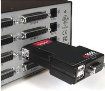
Connect the DB25M connector to the DB25F KVM port on a Rose KVM switch. Next connect your USB keyboard and mouse to the USB Type A connectors on the Uniport. Connect the video cable (HD15M) to the Uniport's HD15F connector.
