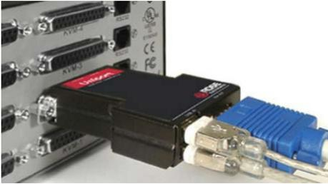
Connect the DB25M connector to the DB25F KVM port on a Rose KVM switch. Next connect your USB keyboard and mouse to the USB Type A connectors on the Uniport. Connect the video cable (HD15M) to the Uniport's HD15F connector.
