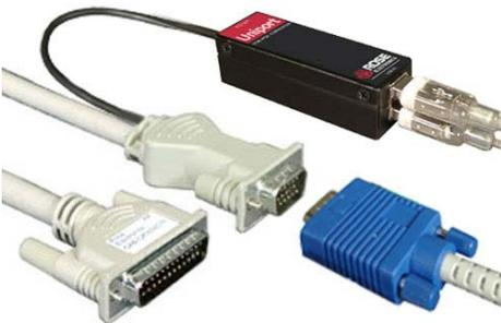
The Uniport "Cable" is a KVM adapter cable. The DB25M connector connects directly to the DB25F KVM port on a Rose KVM switch. The USB connectors and the HD15M connector connect to a KVM stations USB keyboard, mouse and monitor.
