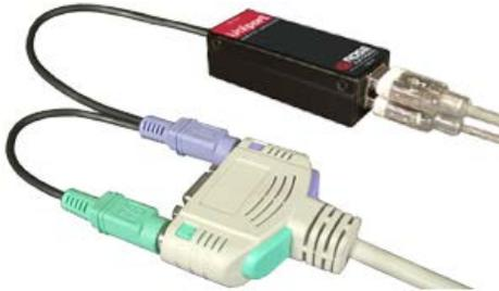
Connect the Uniport's PS/2 keyboard and mouse connectors to the corresponding PS/2 connectors on the KVM cable. Connect the video monitor cable if it was disconnected, to the HD15M connector on the KVM cable. To use a USB keyboard and mouse on a PC, the PS/2 cables can also be connected directly to the PS/2 ports on a PC.
